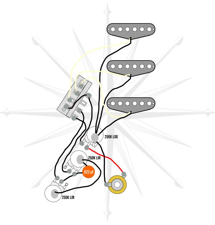
N.B. This diagram is intended to show the signal path of the wiring in this guitar.
